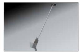
Used to embed DITRA membranes in the bond coat during membrane installation. The lightweight **DITRA-ROLLER** features a 14-1/2" (*37 cm*) wide roller and a shelf for placing 50 to 75 lbs of weight (e.g., bag of thin-set mortar or grout, box of tiles, etc.). Between uses, it can be conveniently disassembled for transport and storage.
