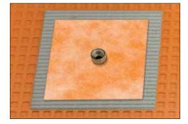
**KERDI-KM** prefabricated seal is cut sections of the KERDI waterproofing membrane designed to seal protrusions through the KERDI or DITRA/DITRA-XL membranes. KERDI-KM is designed to be used in conjunction with Schluter®-KERDI-FIX or equivalent sealant to seal around pipes or other similar elements.
