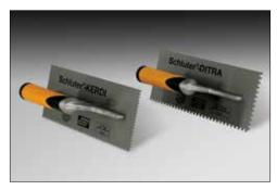
Used to install DITRA and KERDI membranes. The **DITRA-TROWEL** features an 11/64" x 11/64" (4.5 mm x 4.5 mm) square-notched design while the **KERDI-TROWEL** features a 1/8" x 1/8" (3 mm x 3 mm) square-notched design.
