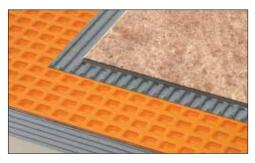
**DITRA-XL** is a pressure-stable polyethylene membrane, vacuum-formed in a cutback grid design, with an anchoring fleece laminated to its underside. DITRA-XL is 5/16" (7 mm) in height and emits zero VOC.
