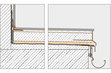
Schluter products make it easy to construct functional balcony coverings that include subsurface drainage, uncoupling/waterproofing, tightly sealed wall joints, and gutters.
