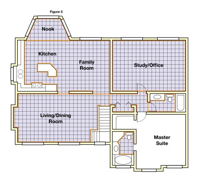
Schluter<sup>®</sup>-Systems understands that the tile setter must take into account the needs of his or her client in determining the placement of movement joints in a tile installation. For example, a client may not wish to interrupt a continuous tile field that spans multiple rooms. However, as indicated by the orange lines above, there are ways to meet industry guidelines that will serve to provide the client with a durable installation that remains aesthetically pleasing.
