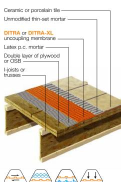
**24**" (610 mm) o.c. joist spacing, double layer OSB or plywood subfloor
